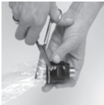
Trimming the excess of the oven tube
