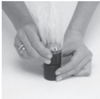
Connecting valve and filling chamber
