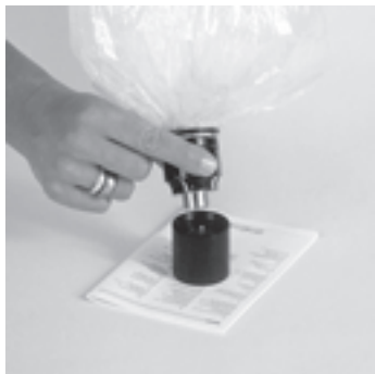
Separating valve and filling chamber
